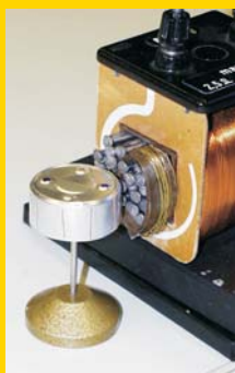
additional winding around the half iron core
