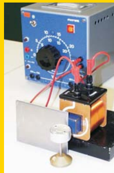
additional winding around the half iron core
